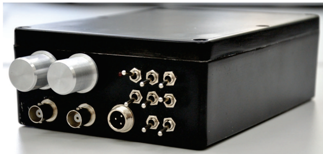
Fig. 13. Designed application board: (top) universal board with components; (bottom) metal enclosure with external terminals
